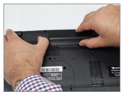
• Pry the battery upward using the indent.
