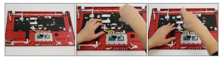
• Remove the five 2.5mm screws by using a Phillips #1 screwdriver.
