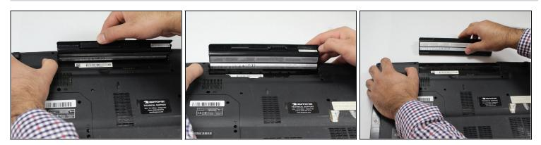
• Continue to pull the battery until it is free of the casing.
