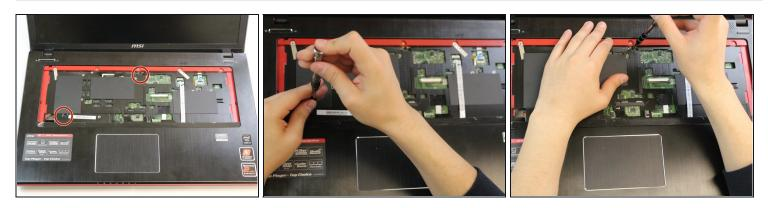
• Remove the two 5.5mm screws by using a Phillips #1 screwdriver.
