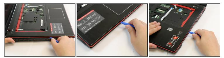
• Using the plastic opening tool, pry open the computer case.
