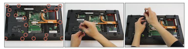
• Remove the twenty-one 5.5mm screws by using a Phillips #1 screwdriver.
