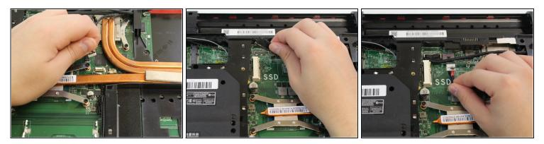
• Disconnect the power, mic, and LVDS cables.
