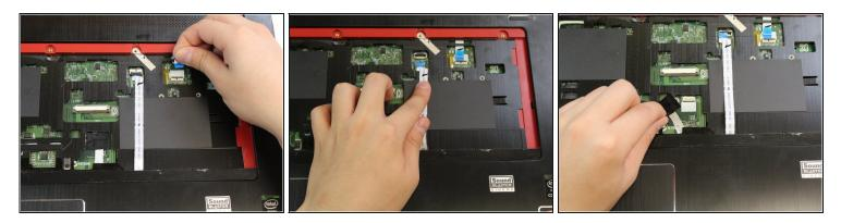
• Disconnect the touchpad, touchpad button, and power board connections.
