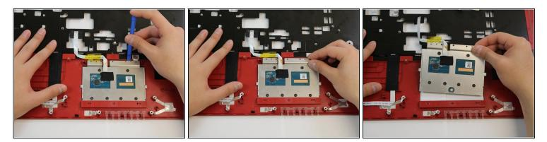
• Using the plastic opening tool, pry the touchpad off and remove it.
