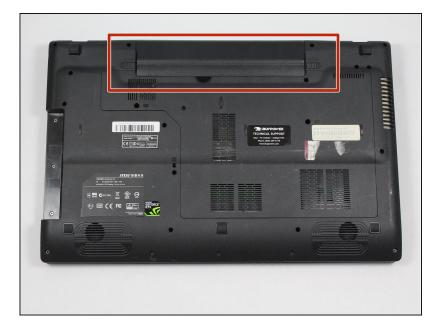
• Turn over the laptop so the battery compartment is facing up.
