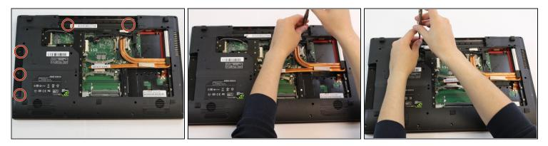
• Remove the five 3.5mm screws by using a Phillips #1 screwdriver.
