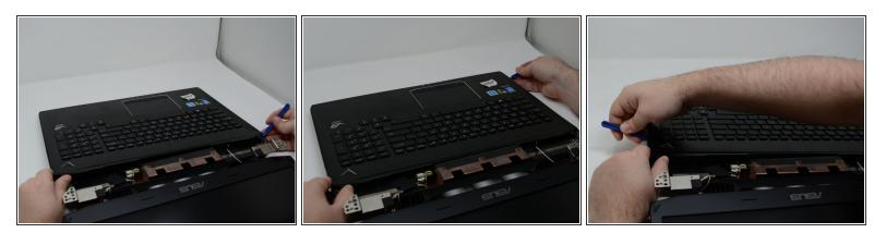
• Pry around the keyboard on the top topside as shown to remove it from shell.
