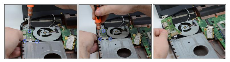
• Remove the three #2 Phillips screws from the small wireless card located in the top left.
