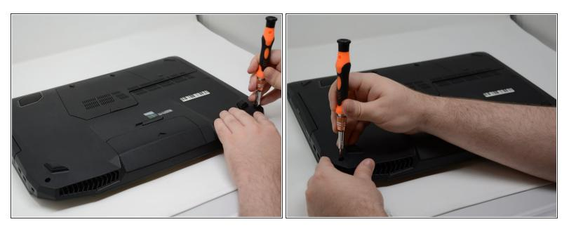
Remove both of the 8mm Phillips #2 screws from these slots where the rubber caps were removed.
