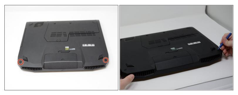
Using a plastic opening tool, remove the two rubber tabs circled in red.
