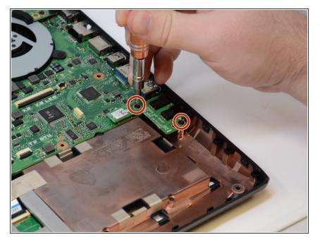
Remove the two #2 Phillips screws for the audio card located in the bottom right.
