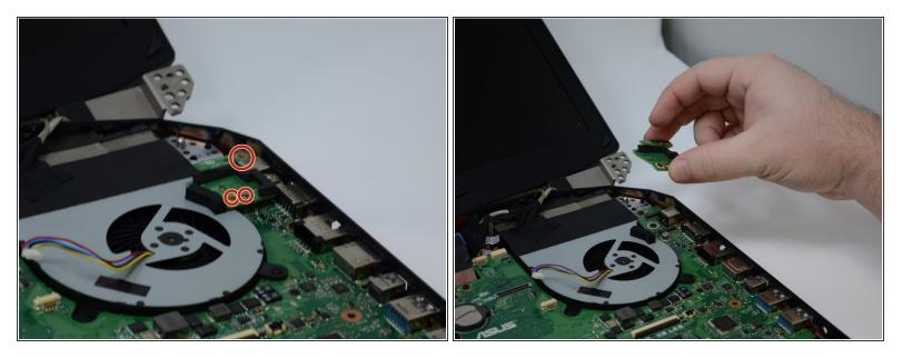
• Remove the three #2 Phillips screws from the small power button card in the top right.
