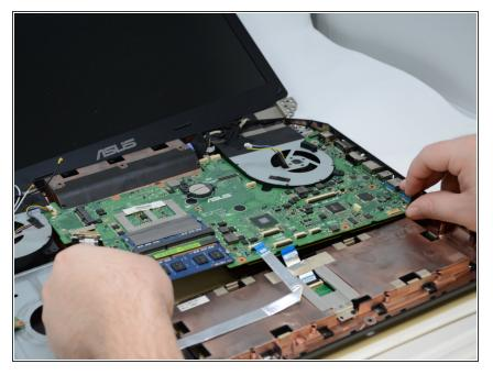
When all the screws are removed, pry up on the edges of the circuit board. You may need your plastic opening tool to access the edges.
