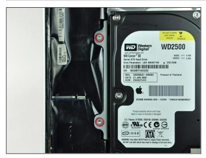
• Remove the two T10 Torx screws securing the hard drive bracket to the inverter.
