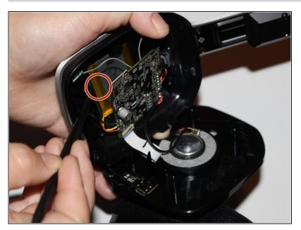
Remove the battery with a plastic spudger.
