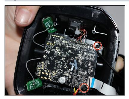
Remove the two 7mm screws with a Phillips #1 screwdriver.
