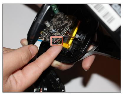
• Lift the motherboard to expose the battery.
