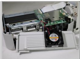
Remove the side panel by lifting it out.
