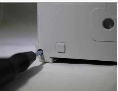
Remove the four 8mm Phillips #1 screws from the bottom of the printer.
