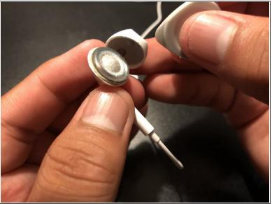
Using a triangle paddle, apply sufficient pressure to get in-between the opening section
