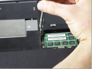
Remove the 7mm Phillips #00 screw from underneath the back panel of the laptop.
