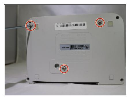
Remove the three 6mm Phillips #1 screws.
