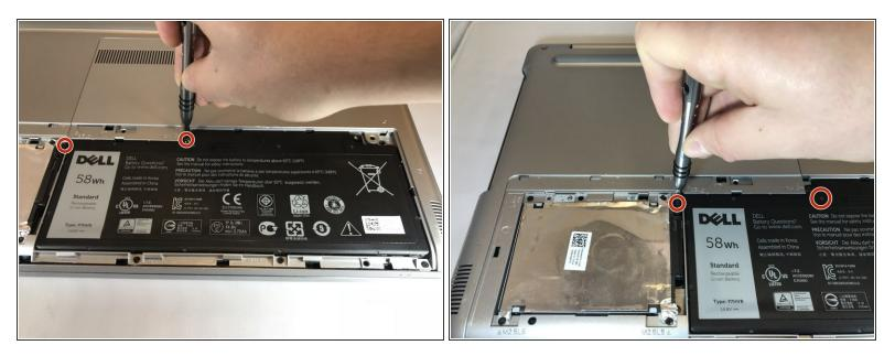
Remove the two black PH1 6mm screws that anchor the battery.
