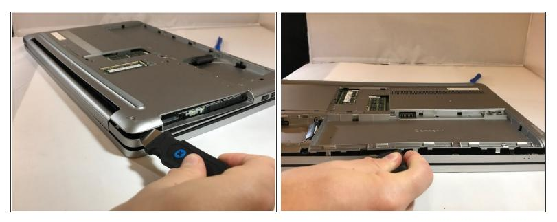
• Close the laptop and flip it over exposing the bottom surface. Use the metal jimmy and blue opening tool, gently pry the bottom cover off. Repeat this process around the entire perimeter of the laptop.
