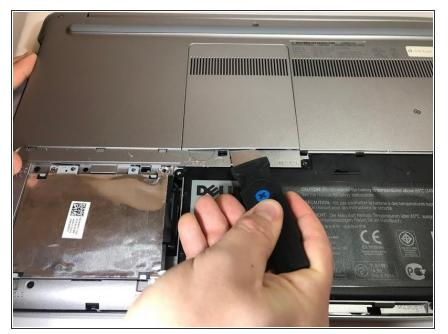
• Pry up the plate covering the RAM, using the metal jimmy.
