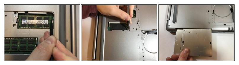
(i) As part of removing all screws the CD ROM screw is also removed using the plastic spudger.
