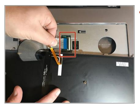
Using your hands, gently remove the wide flat ribbon cable from the motherboard port by gently pulling the cable.
