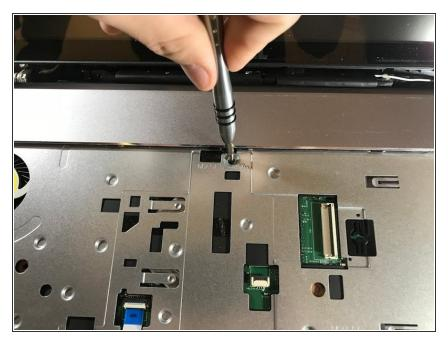
• Remove the 15mm PH 1 screw holding the bottom plate in place.
