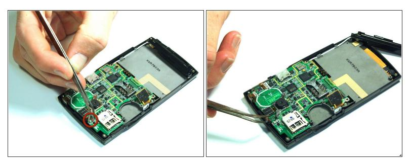
Use the tweezers to unsnap the connection between the motherboard and the speaker. The speaker is attached to the front casing.
