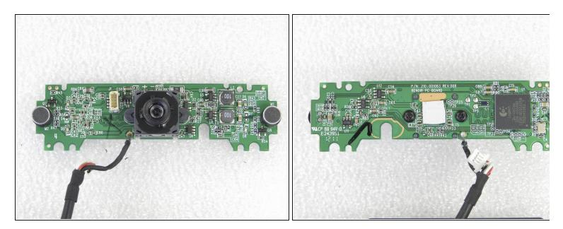
• Front and back images of the webcam's electronic circuit board.
