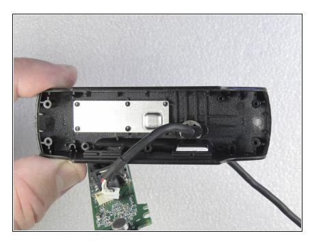
• Remove the electronic circuit.
