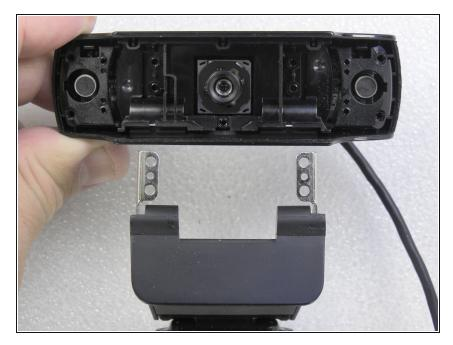
• Carefully remove the metal supports from the webcam's base.
