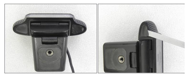
• On the bottom side of the webcam, remove the stickers from both sides
