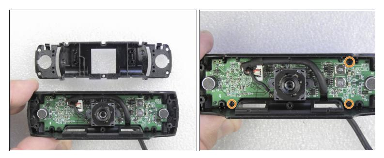
• Carefully remove the base of the plastic support. Loosen the three screws that secure the electronic circuit.
