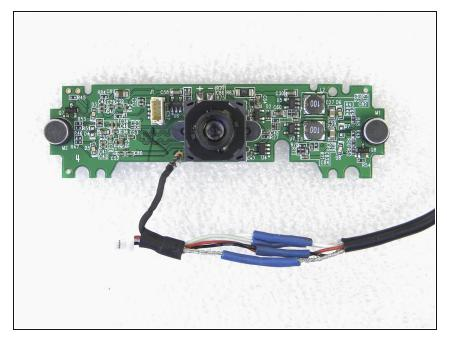
• The problem was the broken cable on the back of the camera. I've cut the faulty part and redid the connections by soldering them and insulated them with heat shrink tubes.
