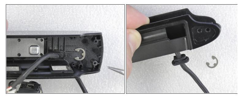
• Release the clip that secures the cable holder. Pull this cable holder out of the camera.
