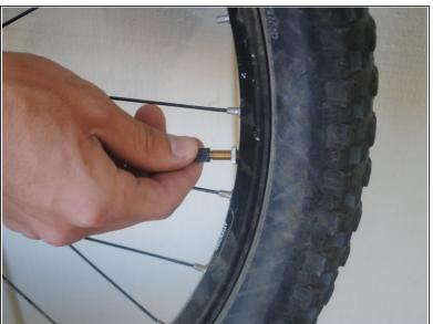
Close the valve and replace the cap.
