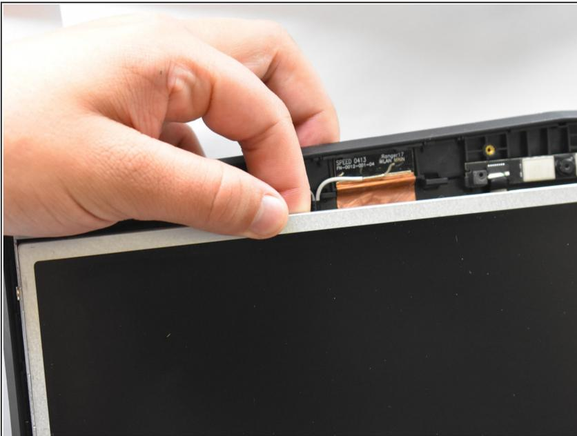
**⚠** Avoid directly touching the connectors with anything other than plastic tools to avoid damaging the internal components.
