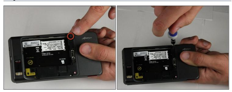
• Identify the screw located in the bottom right corner of the battery case. Remove the screw with a T5 (or in some cases T6) torx screwdriver and set it aside.
