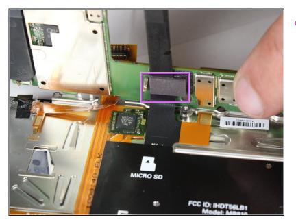
Using the spudger tool, pop the black cable connector off of the motherboard.
