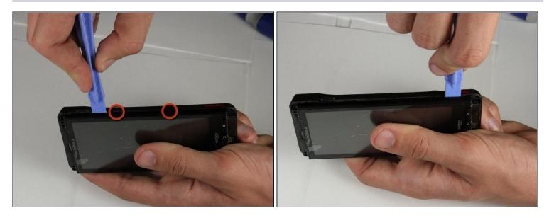
• Locate the seam along the right edge of the phone. Use the prying tool to disconnect the two clips along the edge.
