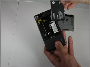
• Find the yellow pull tab located in the upper left corner. Pull the tab until the battery dislodges. Grab the battery by the raised edge, and remove it from the case.
