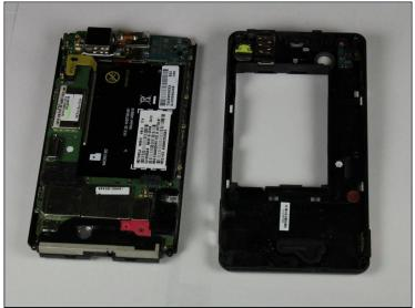
• After the clips are detached, remove the back case and set it aside.
