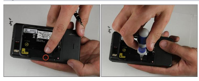
• Flip the phone over and locate the screw on the middle of the left side. Unscrew it using the T5 Torx screwdriver and set it aside.
