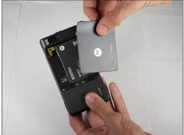
• Place thumb on the back cover, and push down towards the bottom of the device. Once the cover releases, pull it away from the phone and set it aside.
