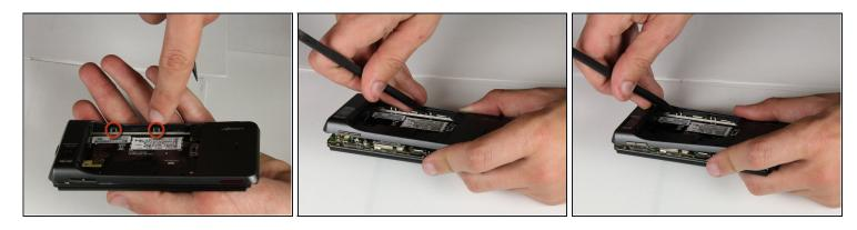
• Locate the two clips on the inside of the case and use the spudger tool to detach them from the case. To detach each clip, use the sharp end to press the small, black plastic in the center of the clip.
