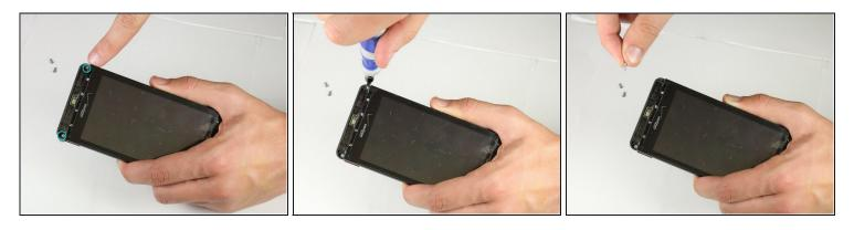
Use a T5 Torx screwdriver to remove the screws in each corner of the phone.
