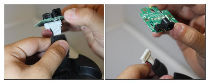
• Pull cable to disconnect board from device.
