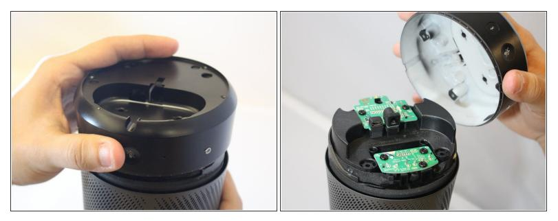
• Firmly grip the bottom and wiggle upwards to remove the base.
