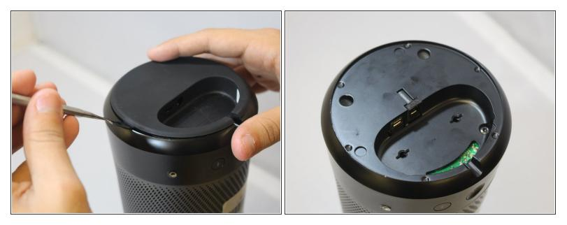
• Use a metal spudger to remove the rubber bottom.
