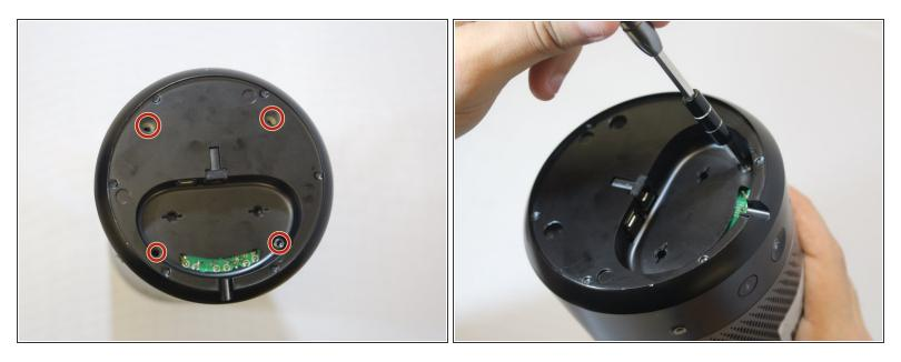
Use a #10 Torx screwdriver to remove four 14 mm screws.
