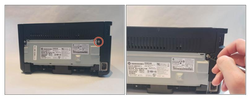
Unscrew the #1 Phillips screw 6mm on the back of the printer.
