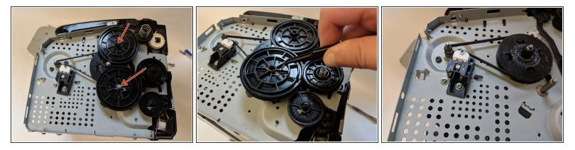
• Remove top two big gears using tweezers.
