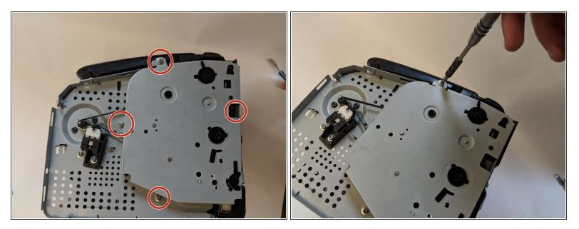
With side panel removed, there will be four Phillips 60mm screws to unscrew using a #1 Phillips screwdriver.
