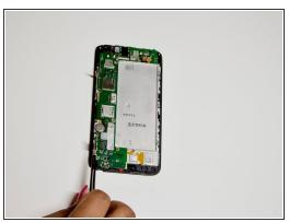
Detach the yellow latches along the sides to remove the motherboard.
