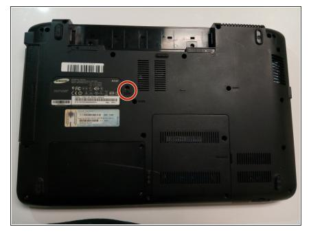
Remove securing screw with the PH0 head.
