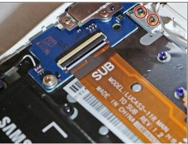
Remove the four 5mm Phillips #0 screws on the hinges.
