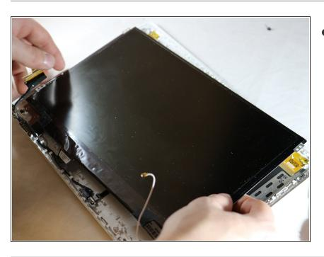
Lift and remove the screen from the device.
