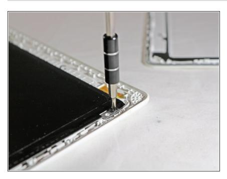
Remove the four 5mm Phillips #0 screws holding the screen in place.
