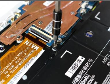
Remove four, 5mm Phillips #0 screws connecting the battery to the laptop
