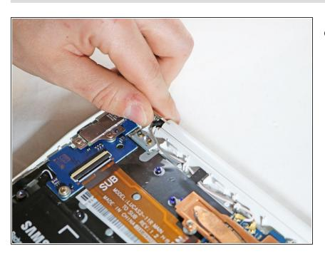
Lift the hinges up and separate the top lid from the bottom casing.
