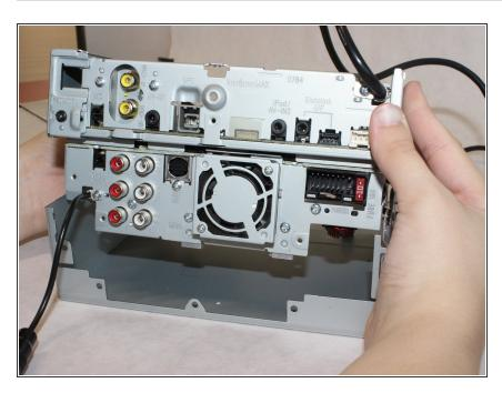
• Lift the top part of the unit up from the lower chassis.
