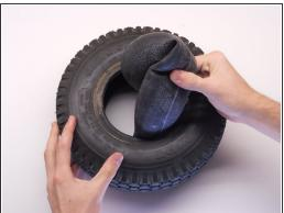
Pinch the deflated inner tube and pull out the inner tube completely.
