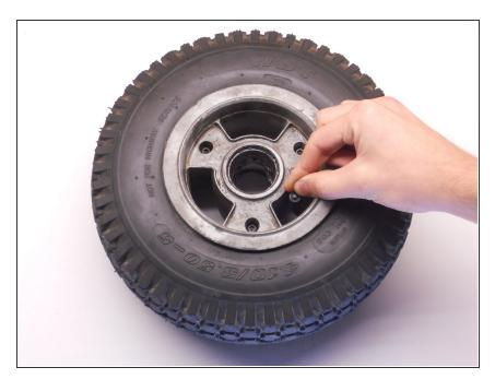
Unscrew the valve cap from the valve stem.
