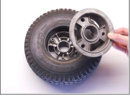
Pull out the rim half that contained the heads of the bolts.
