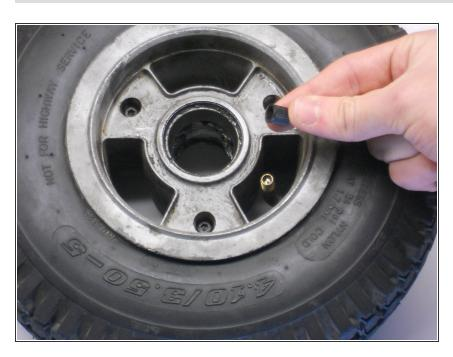
Screw the valve cap onto the valve stem.
