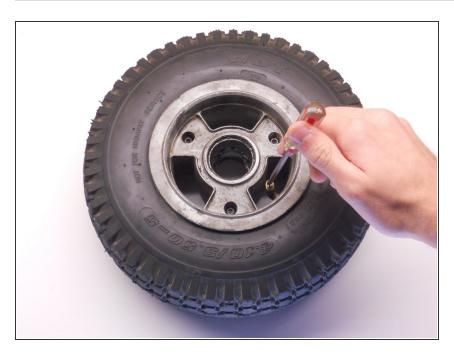
Press the valve all the way down with a screwdriver to release the air pressure.
