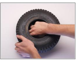
Use two fingers to uniformly push the replacement inner tube into the inside of the tire.
