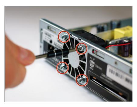
• Use the Torx screwdriver to remove the four 100mm T15 screws.
