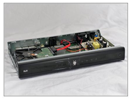
Take the outer casing by sliding the top of the box off of the component carefully, making sure not to damage the surrounding components inside.
