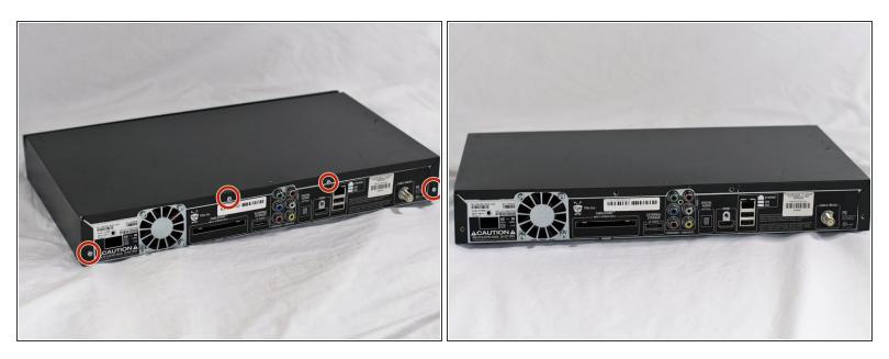
• Remove the four 80 mm T10 screws from the back of the TiVo box using theTorx screwdriver.
