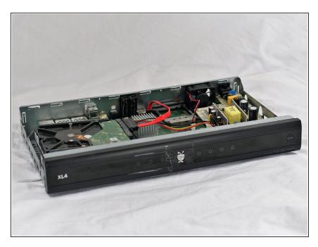
Take the outer casing by sliding the top of the box off of the component carefully, making sure not to damage the surrounding components inside.
