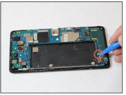
Use a plastic opening tool to unplug the wires by pulling them to the side.
