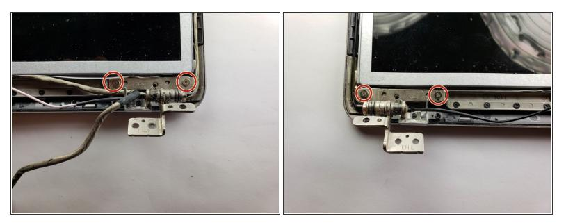
Remove the two 3 mm screws holding the display in place. Repeat this step for both the left and right sides.
