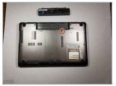
Use the Phillips head screw driver to remove the screw holding the back plate on.
