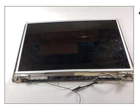
Slide the display upwards to remove it.
