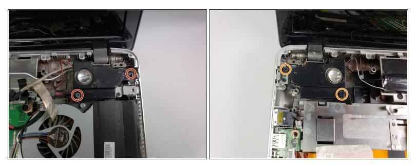
Use the Phillips head screwdriver to remove the 5mm screws on the right speaker.
