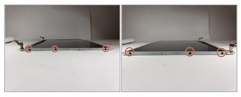
Use the screw driver to remove the six 3 mm screws holding the brackets and hinges onto the display.
