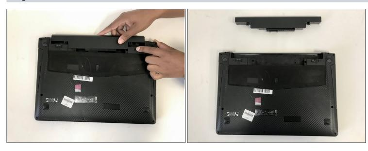
While holding the right battery lock in the unlock position, slide the battery carefully out of the laptop and set it aside.
