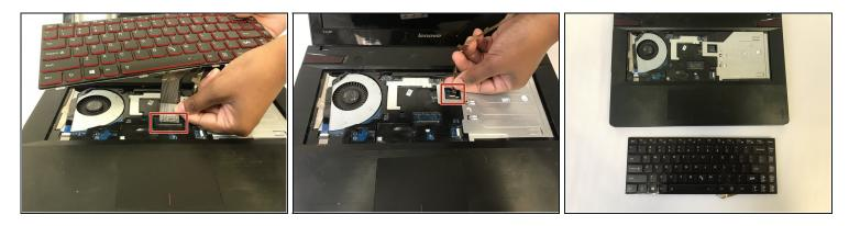
⚠ Be careful when lifting the keyboard so that you do not damage the ribbon cable connector.
