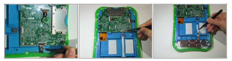
• Remove the ribbon on the bottom of the motherboard and the ribbon on the left side of the motherboard.
