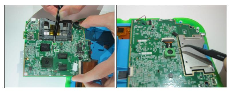
• Flip the motherboard to its back side and pinch the 2 green hooks to remove the camera cover
