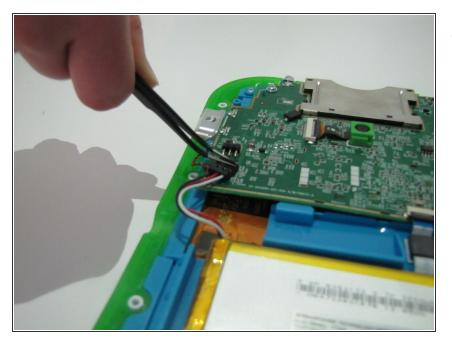
• Remove the 3-pin connector on the top left side of the motherboard.
