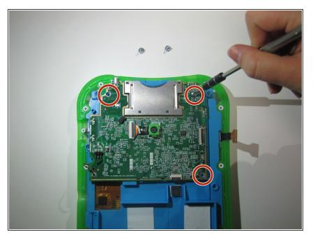
• Remove the 3 screws on each corner of the motherboard
