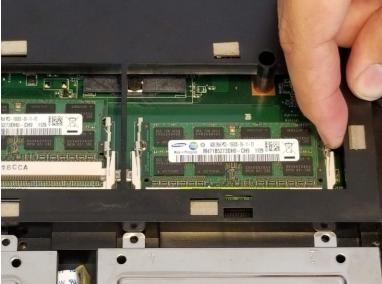
Pry the clips holding the RAM on both sides.
