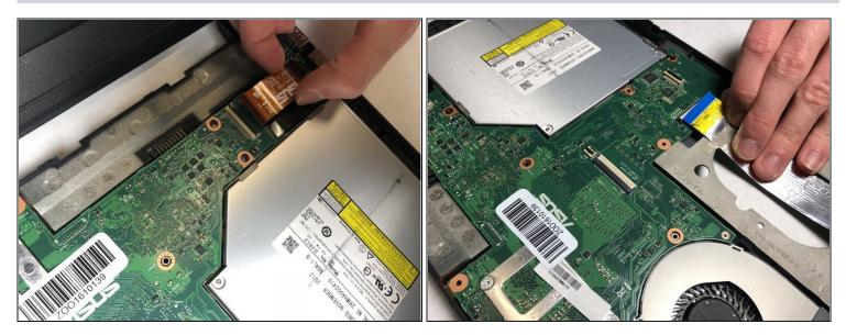
Remove the two remaining ribbon cables as described in Step 7.
