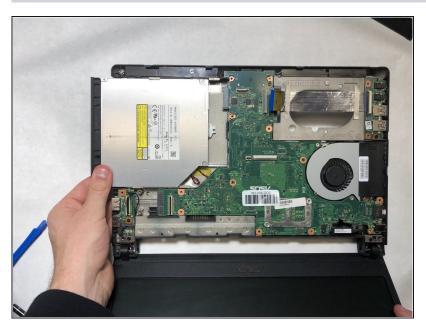
• Firmly grab the optical drive and remove it by sliding it out.
