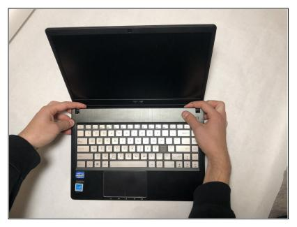
Flip the device right-side up and pry up the keyboard and touchpad gently using both hands.
