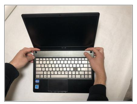
• Flip the device right-side up and pry up the keyboard and touchpad gently using both hands.
