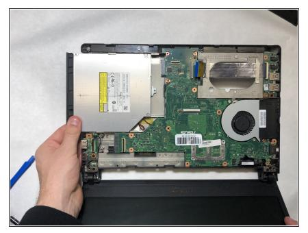
• Firmly grab the optical drive and remove it by sliding it out.
