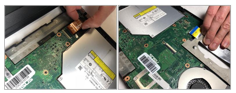
Remove the two remaining ribbon cables as described in Step 7.
