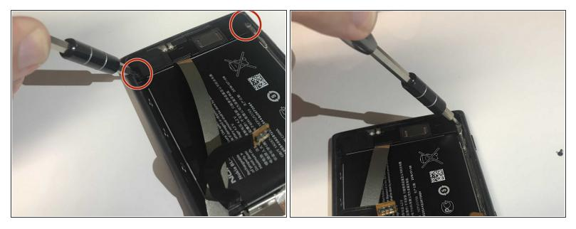
• Remove the two black screws by using the T5 Torx screwdriver.
