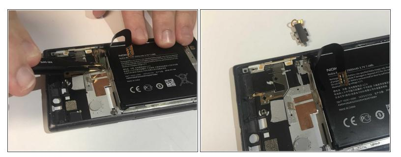
• Pry off the metal vibrating unit using tweezers.
