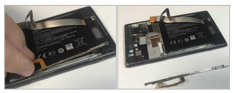
• Carefully pull the metal rod out.
