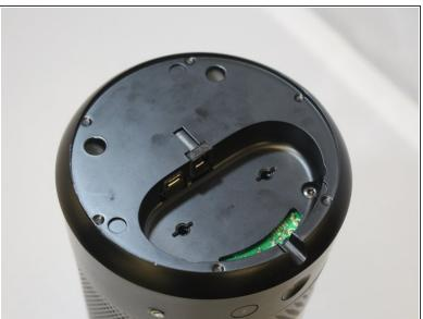
Use a metal spudger to remove the rubber base.
