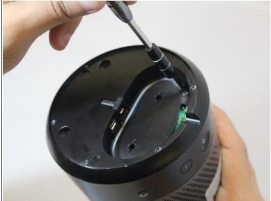
Use a T10 Torx screwdriver to remove the four 14 mm screws.
