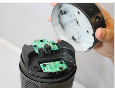
Grip the bottom firmly and wiggle upwards to remove it.
