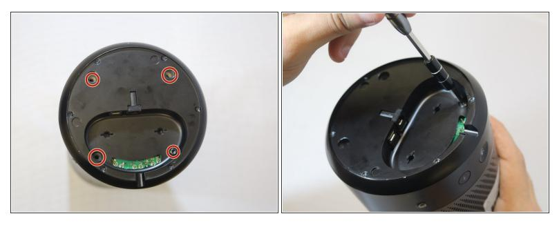
Use a Torx #10 screwdriver to remove the four 14.0 mm screws.
