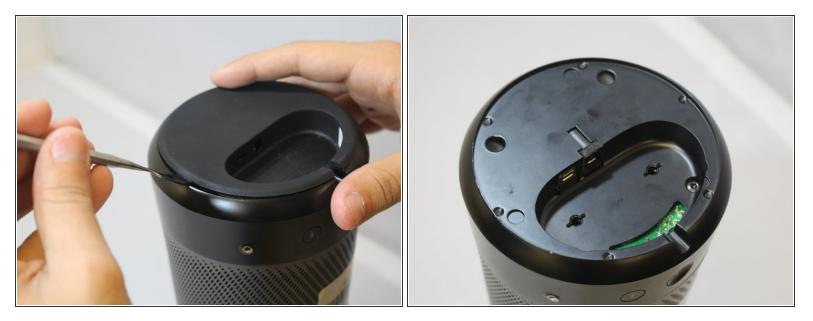
• Use a metal spudger to remove the rubber bottom.
