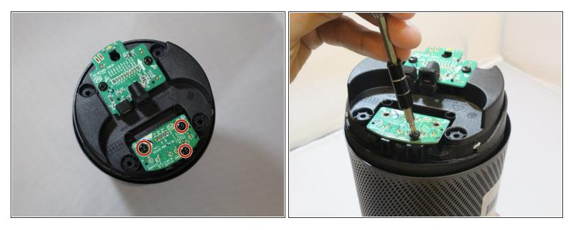
Use a Torx #10 screwdriver to remove three 10.0 mm screws from the highlighted board attached to microphone button.
