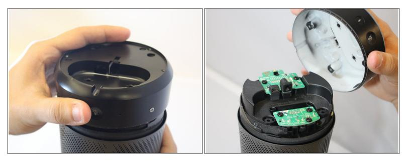
• Firmly grip the bottom and wiggle it upwards to remove the base.
