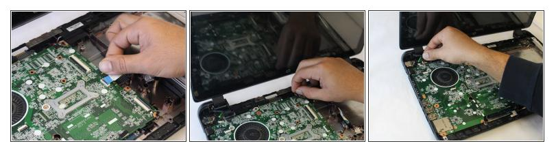
• Locate and disconnect the wires that are connected to the motherboard.
