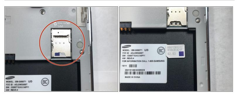
Before disassembling the phone, take out the SIM card and microSD card.
