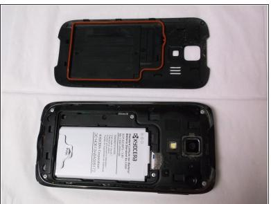
Open the back of the phone by prying the back cover off.
