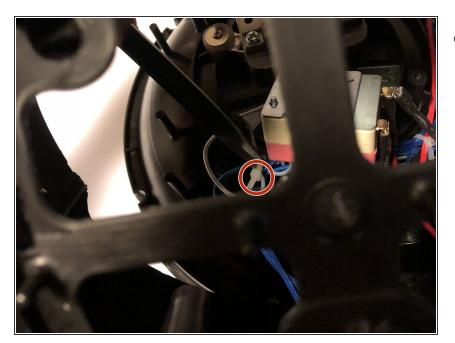
Using a pair of scissors, cut off the cable cord that is securing the wire cords.
