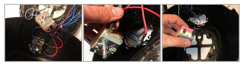
• Detach the device's wires from the potentiometer.
