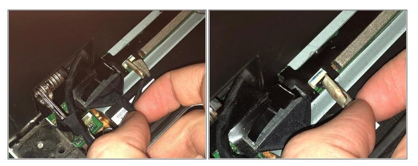
Pull out the 2 wires connecting the monitor to the computer.
