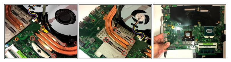
Using a screwdriver with a Phillips #0 head, unscrew the 8 4.2mm screws that connect the heat sink to the motherboard.
