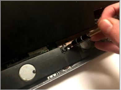
• Use a Phillips #00 screwdriver to unscrew 3 screws on the audio board.
