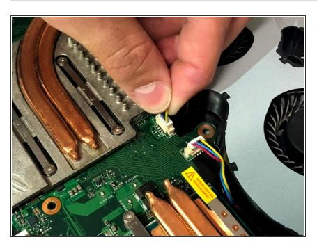
Disconnect the 4 Pin Connectors from the motherboard.
