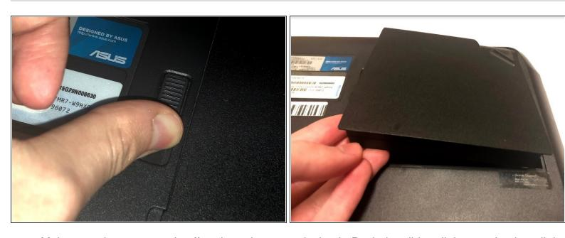
Make sure the computer is off and turn it over on its back. Push the slider all the way back until the compartment for the battery opens. Remove the battery and place it aside.
