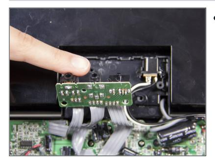
• Pull out the AV circuit board and lift it up and out of the way to allow access to other components.
