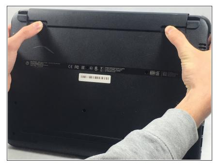
• Remove battery by pushing the two buttons inward.
