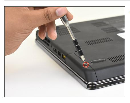
Use a Phillips #00 screwdriver to remove one M2 x 3mm screw from the side of the device.
