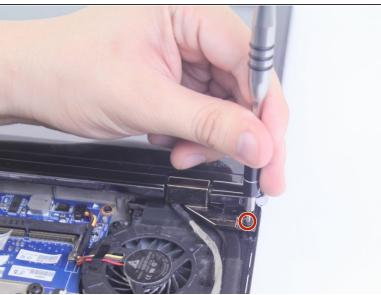
Unscrew the two M2 x 3mm screws near the hinges using a Phillips #00 screwdriver.
