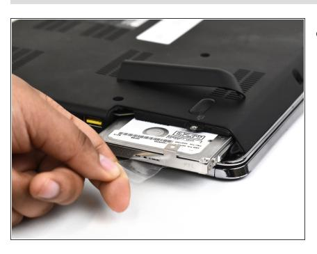
Use the clear tab to slide the hard drive out of the device.
