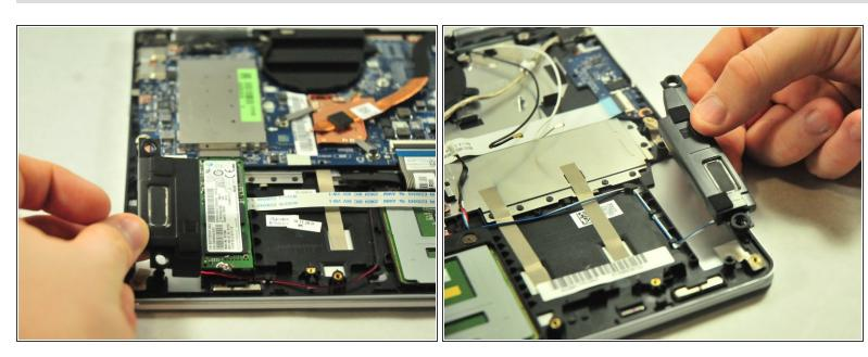
Untangle the wires from the plastic hinges of the case to properly lift the speakers out.
