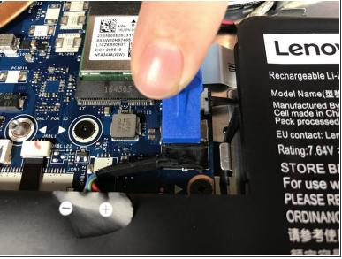
• Use your fingers or an opening tool to slide the battery connector out of its motherboard socket.
