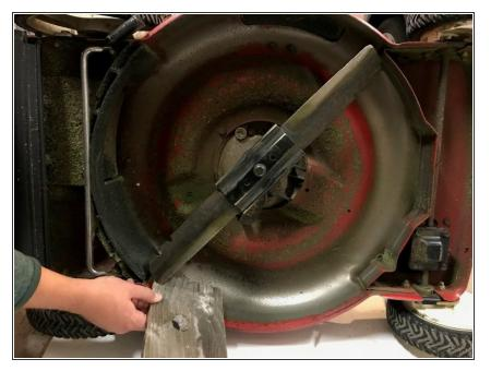
Place wood in between the blade and the wall of the mower to ensure that the blade does not move while you are tightening or loosening the bolt.
