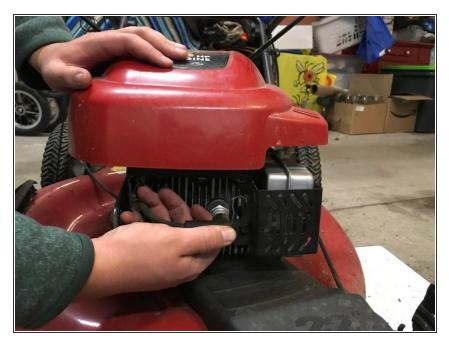
• Flip the mower right-side up and reconnect the spark plug.
