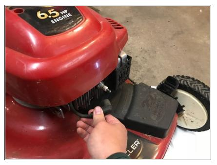
Disconnect the spark plug to ensure that the lawn mower does not accidentally turn over and cause the mower to turn on.
