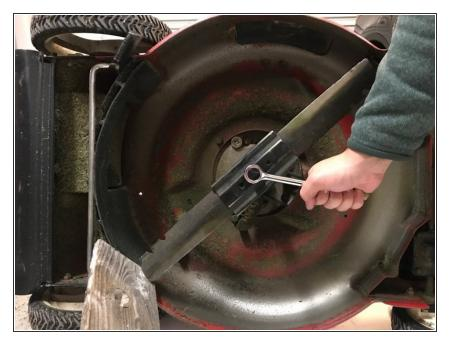
• Using the 5/8 ratchet, turn the bolt clockwise until the bolt does not turn anymore.
