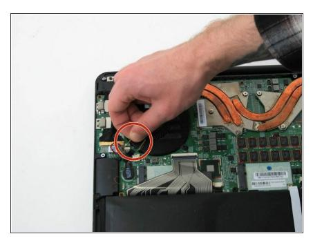
Disconnect the wire that goes from the fan into the white connector, but leave the wire attached to the fan.
