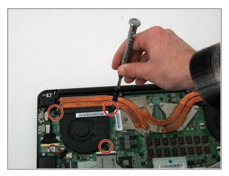
Use the Phillips #0 screwdriver to remove the three 1/4 inch screws.
