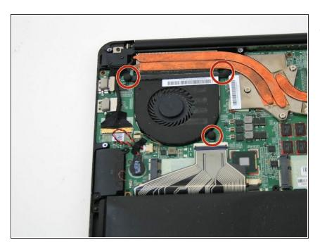
Remove the three black rubber pads that cover the screws holding the fan.
