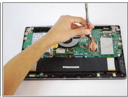
Using a Phillips #1 Screwdriver remove the three 3 mm black screws and four 2 mm copper screws holding the fan and heat sink in place.
