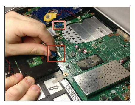
Disconnect the motherboard from the two connectors shown.
