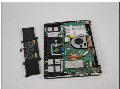
Gently remove the battery from the slot.
