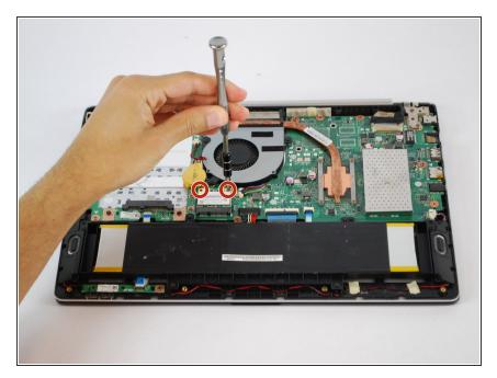
Using a Phillips #1 Screwdriver unscrew the 2 mm screw holding the wifi card in place.
