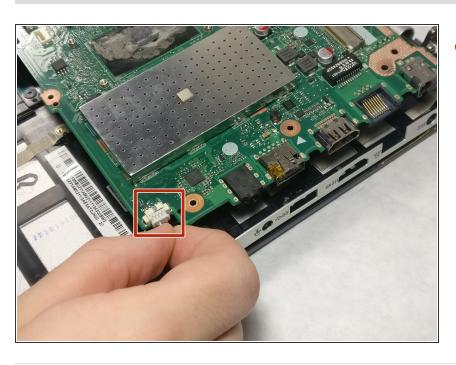
Disconnect the motherboard from the connector shown and it is now removed from your device.
