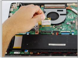
Unplug the Wi-Fi card from the motherboard and remove it from the device.
