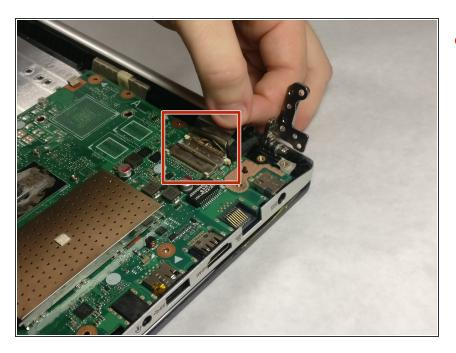
Disconnect the motherboard from the connector shown.
