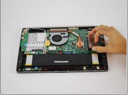
Remove the top covering the RAM chips.
