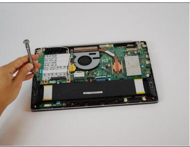
Using a Phillips #1 Screwdriver remove the six 3 mm screws keeping the battery in place.
