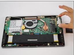
Remove the RAM from the device.
