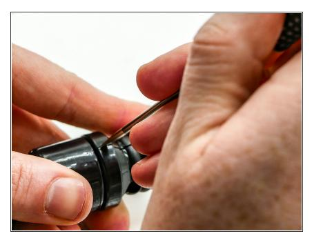
Use a flat head screwdriver to assist in prying open the plastic housing.
