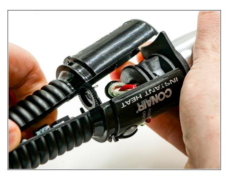
Gently open the plastic housing making sure to evenly pull apart the plastic so it does not bend or snap.
