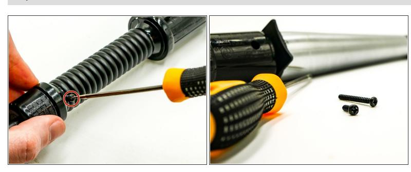
Remove the next 4 mm screw with a Phillips #0 screwdriver.
