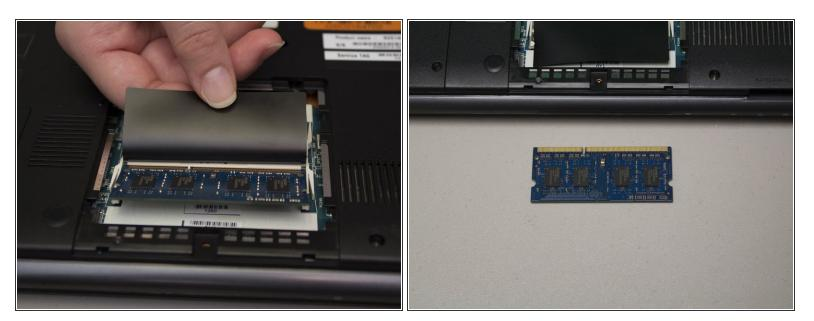
(i) Once both anchors are released from the RAM stick, the stick will spring up at an angle
