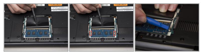
With the cover removed, peel back the black protective plastic to expose one of the two RAM sticks.
