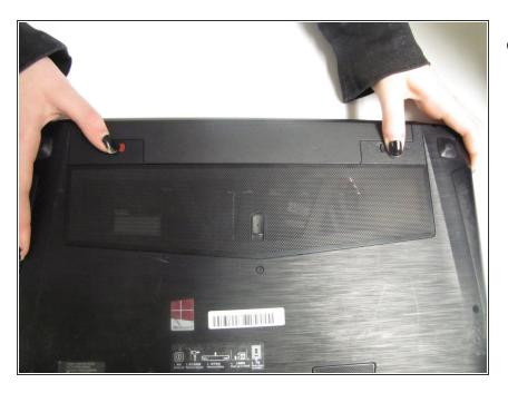
Move latches to the unlocked position.
