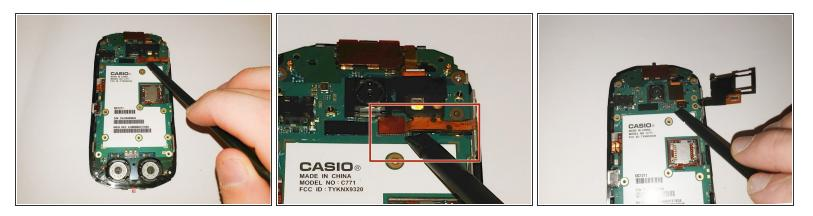
• Using a spudger, gently lift up the orange connector.
