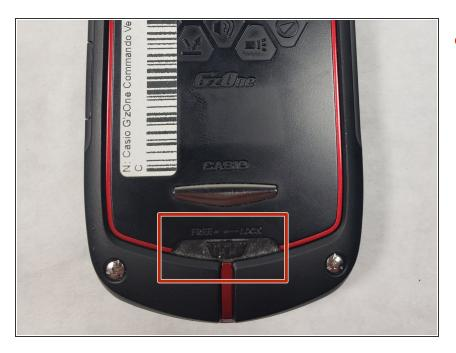
• Slide the slider on the back of the phone to the free position.
