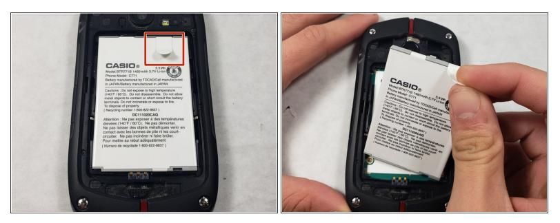
• Pull the white battery tab upwards and remove the battery.
