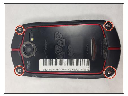
• Remove the four 5mm Y0 screws from the back of the device.
