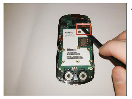
Using a spudger, pry away the motherboard from its compartment, by inserting the spudger in the compartment and lifting upwards until fully out.
