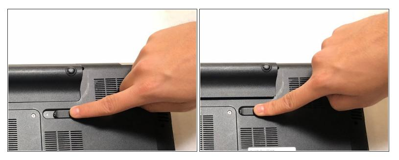
Slide the battery release switch to the left. The battery pack will then subsequently release.
