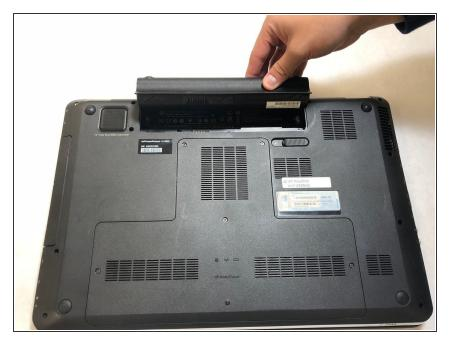
Remove the battery pack from the socket.
